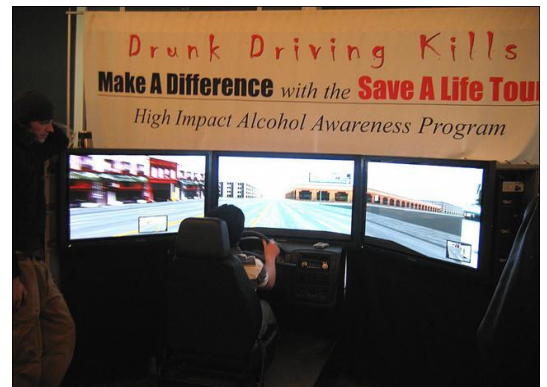
Brian Beldyga, a senior manager with the entertainment group who provided this simulator, is explaining the mechanical delay between when you turn the wheel and when the “car” reacts. That delay simulates the chemical one in the brain when you drink, he said. About 150 Thiel students tried out the simulator on Wednesday in the Howard Miller Student Center.
